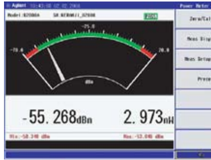
N9340B supports Meter and Chart mode to display the results of power measurements.
