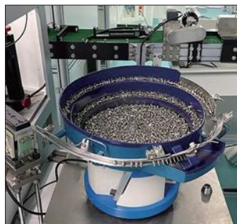
vibratory feeder loading
