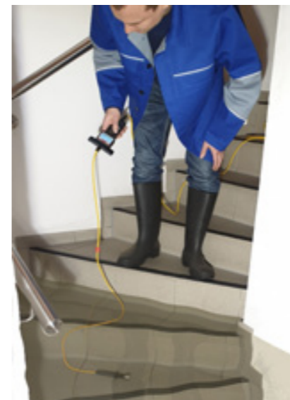
The ball electrode probes voltage in the water from a safe distance
