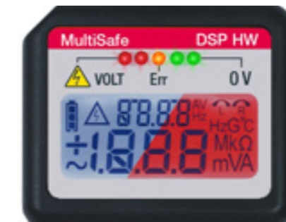
Display with bright LEDs and two-color LCD
