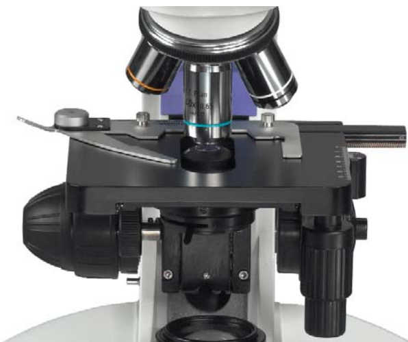
Plan achromat objectives are parfocal and parcentred to minimise refocusing.
