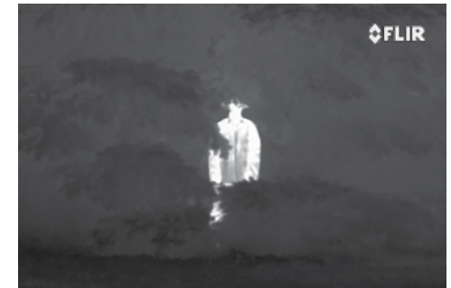
Thermal imaging: person hiding in bushes is clearly visible since thermal contrast is practically impossible to mask.
