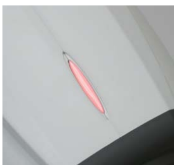
LED irradiator to visualize the discharge (Change the color from red to green upon the discharge)
