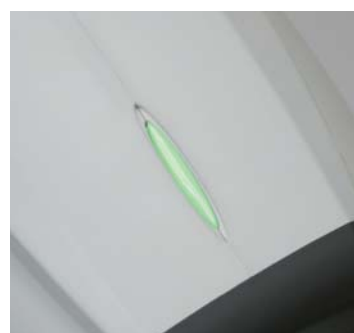
LED irradiator to visualize the discharge (Change the color from red to green upon the discharge)
