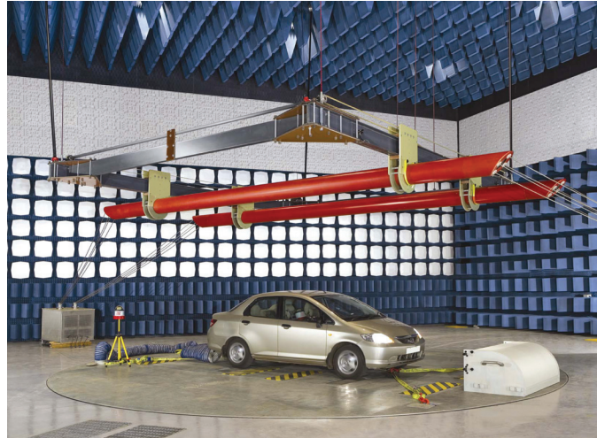
ETS-Lindgren's Model 5502 with Optional 8 m Long Elements (4340 Shielded CCTV Camera Not Included)
