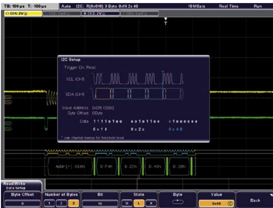
Decoded hexadecimal I 2 C message.
